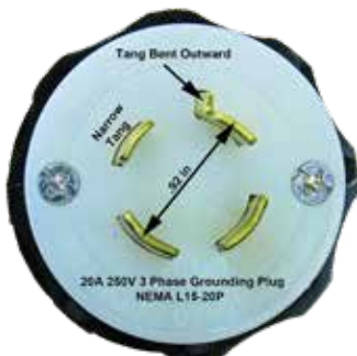
20A 250V 3PH Grounding Plug (NEMA L15-20P)
