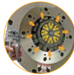
Easy grease maintenance through the 8 lubrication fittings
