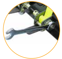
Quick tightening using the wrench and quick release using the quick release pedals
