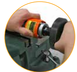
Change from OD to ID skiving tool in seconds with PTO coupling
