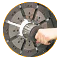
Quick change tool makes die changes a quick and simple process
